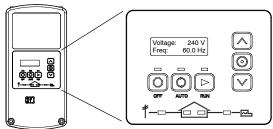
The RDC2 controller provides integrated control for the generator set, Kohler<sup>®</sup> Model RXT transfer switch, programmable interface module (PIM), and load shed kit.
